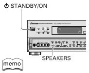
To check which impedance setting to hold down the SPEAKERS button for 2-3 seconds. You'll get a display like these telling you the speaker impedance setting.
